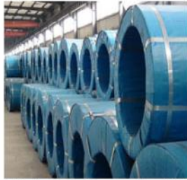
Each Coil is Strapped by steel bands at 8 places, fully wrapped with anti-rust plastic & P/P woven
