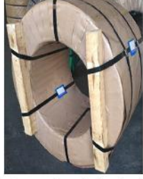
Sheet with pallet and strapped again by steel bands at 6 places.
